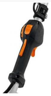
Stihl Ecospeed – With the ECOSPEED function, you can use your long reach hedge trimmer in a more economical operating mode. Simply turn the wheel to the minus direction, thereby reducing the maximum engine speed. This keeps your long reach hedge trimmer running at partial load; however, despite this limited setting, you can shift to full capacity when necessary by pressing the throttle lever. Operating at partial load reduces fuel consumption and you can work much longer with one tank.
