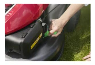
Versamow – With a single lever, Honda's Versamow system will collect the grass cuttings into the bag or finely shred and blow them down into the lawn to create a natural fertiliser or the perfect mix of both
