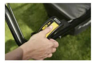
Roto-stop - Stops the blades but leaves the engine running while you empty the grassbag or move across driveways with self propelled models
