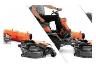
XChange - Unique quick coupling allows attachments to be changed quickly and easily without the need for any tools. Get ready for a new task in just a minute.
