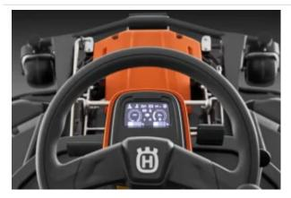
HMI Display - The intuitive display communicates with the driver through visual symbols and warning sounds, assists in handling and gives real time data and warnings.
