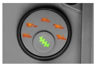
Non-collecting mode - Easy switch between collecting and non-collecting mode by just pushing a button. You don't have to leave the driver's seat.
