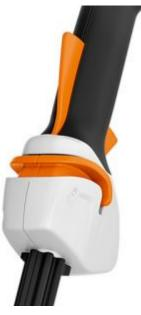
Ergonomic Control Handle - The FSA 60 R has a locking lever (orange front), ERGO lever (black) and main trigger lever (orange below). The locking lever is self-resetting and prevents unintentional switching on of the device. When the ERGO lever and shift lever are pressed, you can work continuously with ease.
