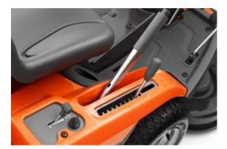
Easy-access cutting height lever - The cutting height lever is easy to reach from the driver's seat, making it possible to do cutting height changes while mowing.
