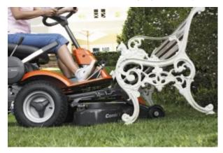
Front-mounted cutting deck - Front-mounted cutting deck for excellent accessibility into corners and under bushes, park benches etc.
