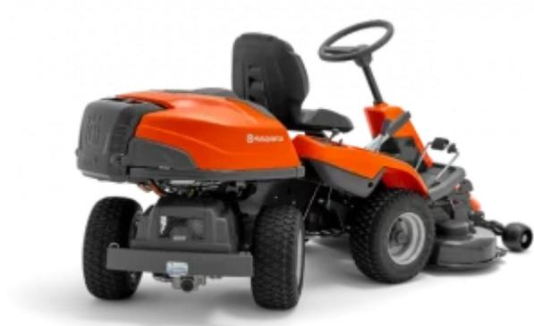
**All-Wheel-Drive (AWD)** - All-Wheel-Drive (AWD) ensures traction on uneven, wet and slippery areas and slopes. AWD automatically adjusts the traction on all wheels depending on situation and ground condition.
