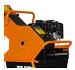
Low Noise - In the interests of the environment, ELIET always try to obtain harmony between the machine and its surroundings. The shredding chamber has a double wall in order to reduce the noise pollution from this chipper. The frame wall sound damping material dampens the drumming effect of the chippings on the wall. This action reduces the noise level by several dB.
