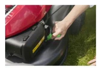
Honda Versamow - With a single lever, Honda's Versamow system will collect the grass cuttings into the bag or finely shred and blow them down into the lawn to create a natural fertiliser or the perfect mix of both.
