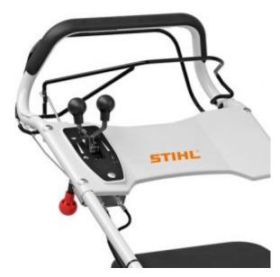
3-speed gearing and Blade Brake Clutch - The blade brake clutch disengages the blade and engine to protect the crankshaft. This allows the grass catcher box to be emptied without restarting the engine. The mower can also be driven around the garden without the blades working. The mowers drive speed can be controlled by means of three forward gears.
