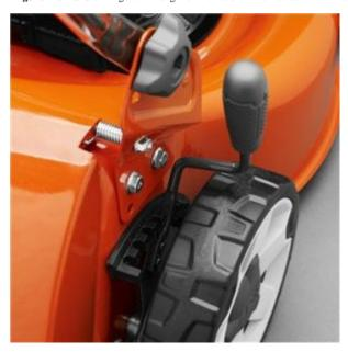
Central cutting height adjustment - Quick and easy adjustment of the grass cutting height. One lever controls the whole deck.
