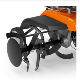
**Dividable hoe set** - The dividable hoe set accompanying this STIHL tiller allows the variable adjustment of the working width. As a result, crops can be planted in rows close to one another. The lateral discs protect existing plants from sustaining damage during tilling.
