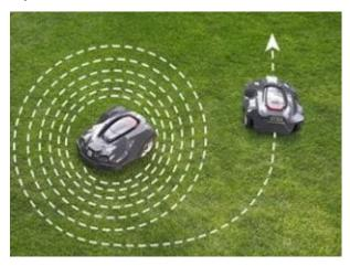
**Spiral Cutting** - Automatic cutting functionality to even out grass height differences. Cutting disc sensors detect whether the mower enters area with higher grass and switches cutting technology to systematic spiral pattern.
