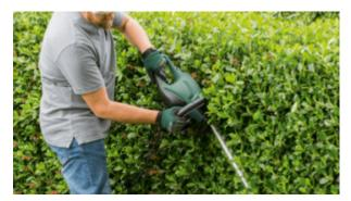
Laser-cut, diamond-ground blades for cutting 26mm wide branches quickly.
