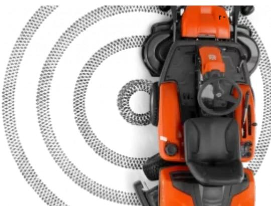
**Unique Articulated Steering** - The unique articulated steering system allows the rear pair of wheels to swing in underneath the machine. The result is superior manoeuvrability with a minimum turning radius at full lock.
