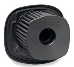
**HD2 Filter** - The HD2 filter, made from polyethylene filter material, has pores that are up to 70% finer than those of fleexe and polyamide filters and therefore eliminates even the finest dust. In addition, it repels oil and water and is therefore very easy to clean. The PET filter cartridge can be removed and inserted without tools.
