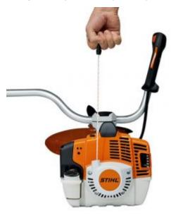
Stihl Ergostart - STIHL ErgoStart cuts the effort required to start the tool by half, while the starter cord can be pulled at just one third of the normal force. A coil spring between the starter cord and the crankshaft smoothes out force peaks, making them virtually undetectable through the cord itself.
