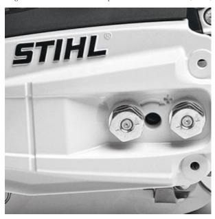
Side chain tensioner - The tensioning screw can be found on the side of the chain saw through the sprocket cover. This removes the need for contact with the sharp saw chain.
