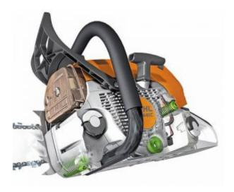
Anti-vibration system - Intense vibration at the handles of power tools can lead to long-term effects on blood vessels in the hands and arms. STIHL has therefore developed an effective anti-vibration system whereby the oscillations from the machine's engine are dampened which significantly reduces vibrations at the handles.
