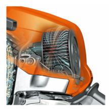
HD2 Filter - The HD2 filter is made from polyethylene filter material with up to 70% finer pores than fleece and polyamide filters to trap even very fine dust. In addition, it is oil and water-repellent and thus very easy to clean. The PET-covered filter cartridge with quick-release lock enables the filter to be assembled and disassembled in next to no time, without using tools.
