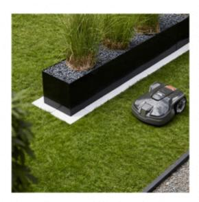
Automatic passage handling – PATENTED – Husqvarna Automower® automatically senses narrow passages and finds its way even through the smallest passages. It will vary its route through the passage to avoid unpleasant tracks.
